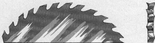
all-purpose rip and crosscut circular saw blade
